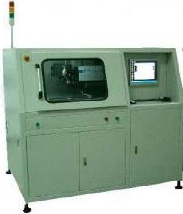
50 Watt Nd:YAG Laser with X-Y-Z programmable axis
